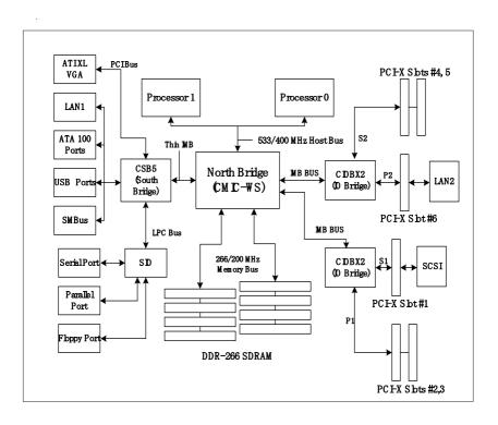
Figure 1-5. ServerWorks Grand Champion LE Chipset: System Block Diagram
